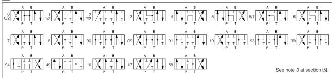
DKI,DKU and DKOR are spool type, three or four way, two or three position direct operated solenoid valves designed to operate in oil hydraulic systems.
